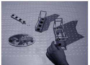
Figure 1: "Urp" urban planning simulation, with buildings, wind tool, and wind probe
