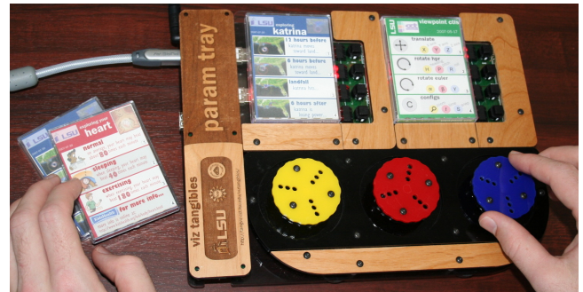
Figure 1. Tangible menus and interaction trays: several data and parameter menu cards are shown with a three-wheeled parameter tray
