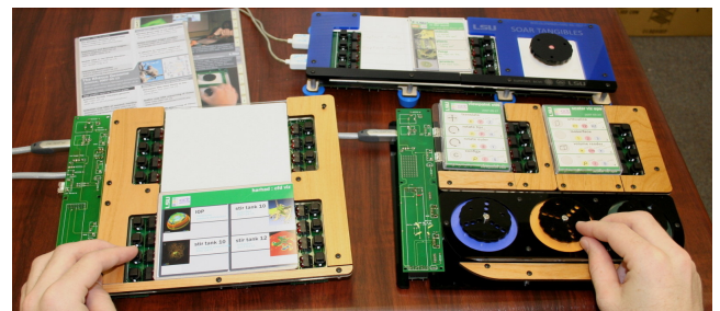
Figure 3. Several tangible menus and interaction trays. From top right: application tray; param tray w/ two param cards; menu tray w/ short menu
