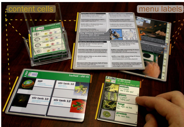
Figure 2. Tangible menus: clockwise from top-left, parameter cards in card deck; data menus; data menu card; and short data menu
