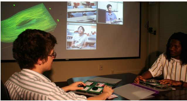
Figure 5. Co-located and distributed users collaboratively manipulate a visualization application in an AccessGrid meeting room. Four interaction trays (two local, two remote) are used with tangible menus to load and save data, manipulate parameters, etc.
