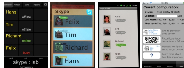
Figure 2. Three editions of smartphone cartouches. Screens are in the context of the Skype teleconferencing example. a) Existing TouchOSC app, implemented with several container and tool templates; here with four slots bound to people, displaying their Skype status. b, c) Google Android and Apple iOS apps implementing the same functionality, augmented with image labels. d) Prototype network configuration screen.
