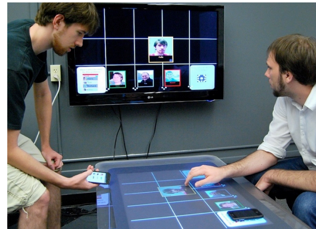
Figure 1. Smartphone cartouches used with Microsoft Surface and wall display. Two smartphones – one Android, one iOS – are used as “containers” for Skype (voice/video/chat) handles to people. Each smartphone employs native apps communicating via the OSC protocol. The location within the Surface’s grid where these are placed, and how they are manipulated, controls which actions and mediations are executed.
